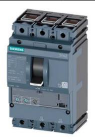
CIRCUIT BREAKER 3VA2 IEC FRAME 160 BREAKING CAPACITY CLASS L ICU=150KA @ 415 V 3POLE, LINE PROTECTION ETU320, LI, IN=160A OVERLOAD PROTECTION IR=64A ...160A SHORT CIRCUIT PROTECTION II=10 X IN CABLE CONNECTION
