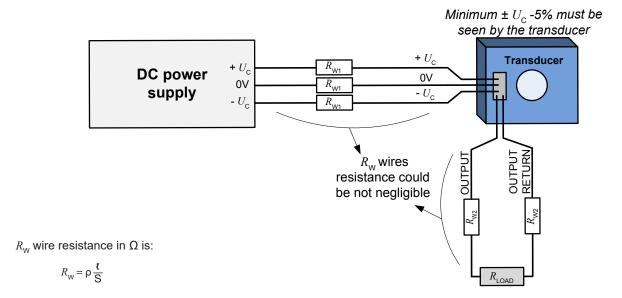
S: Cross section of wire in m<sup>2</sup>
