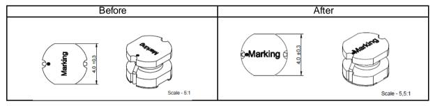
3. The marking and start of winding indication (dot) in the packaging drawing will be turned by 90° for sizes 4532, 5820, 5848, 7850, 1054 and 1065
