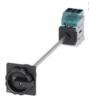
Switch disconnector 3LD3, main switch 3-polig, lu 40A operational switch at AC-23 A at 400 V 15,0 kW floor mounting Base mounting with door coupling center-hole 22,5 mm rotary operationg mechanism black 66 x66 mm
