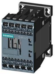
CONTACTOR RELAY, 3NO+1NC, AC 110V, 50/60 HZ, SZ S00, SPRING-LOADED TERMINAL
