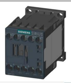
COUPLING RELAY, AC-3, 3KW/400V, 1NC, DC 24V, 0.7...1.25\*US, W. INTEGR. SUPPRESSORDIODE, SZ S00, SCREW TERMINAL
