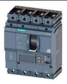
CIRCUIT BREAKER 3VA2 IEC FRAME 160 BREAKING CAPACITY CLASS M ICU=55KA @ 415 V 4POLE, LINE PROTECTION ETU560, LSIG, IN=160A OVERLOAD PROTECTION IR=64A ...160A SHORT CIRCUIT PROTECTION ISD=0,6..10X IN, II=1,5..10X IN NEUTRAL PROTECTION ADJUSTABLE (OFF, UPTO 100%) GROUNDFAULT, SWITCHABLE IG=0,2... 1 X IN, TG=0,050,8MS BUSBAR CONNECTION
