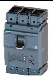
CIRCUIT BREAKER 3VA2 IEC FRAME 400 BREAKING CAPACITY CLASS H ICU=85KA @ 415 V 3-POLE, LINE PROTECTION ETU860, LSIG, IN=400A OVERLOAD PROTECTION IR=160A ...400A SHORT CIRCUIT PROTECTION ISD=0,6..10X IN, II=1,5..10X IN NEUTRAL PROTECTION OPTIONAL WITH EXT. CT;UPTO 160% GROUND-FAULT, SWITCHABLE IG=0,2... 1 X IN, TG=0,05-0,8MS BUSBAR CONNECTION
