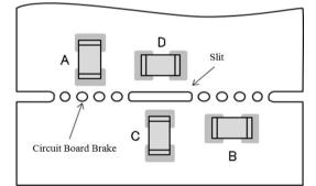
Stress strength according to the mounting position: A > B > C > D
