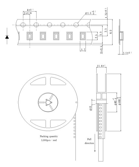
(Unit : mm) (Note) Tolerance is within ±0.2mm unless otherwise specified.
