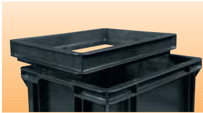
Extension frame to increase useful container height by 44 mm. Fixed to container by Nylatches or U-clips. Available in two sizes: 600 x 400 and 400 x 300 mm.
