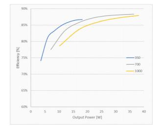
OTI DALI 40 NFC LP Typical Efficiency vs. Load (230 V 50
