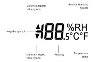
The LCD shows six different recorded readings, which can be cycled through using the built-in push button. The most recent logged value, maximum logged value and minimum logged value can be displayed separately for humidity and temperature. In addition, logging and alarm status is shown using two high intensity LEDs.
