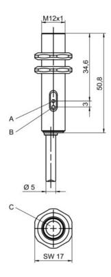
A Green LED B Yellow LED C Optical axis Part no.: 50140158 – LE412B/2 – Throughbeam photoelectric sensor receiver
