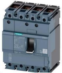
CIRCUIT BREAKER 3VA1 IEC FRAME 160 BREAKING CAPACITY CLASS S ICU=36KA @ 415 V 4-POLE, LINE PROTECTION TM210, FTFM, IN=125A OVERLOAD PROTECTION IR=125A FIXED SHORT CIRCUIT PROTECTION II=10 X IN NEUTRAL UNPROTECTED BUSBAR CONNECTION
