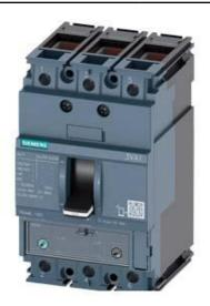
CIRCUIT BREAKER 3VA1 IEC FRAME 160 BREAKING CAPACITY CLASS N ICU=25KA @ 415 V 3-POLE, LINE PROTECTION TM240, ATAM, IN=25A OVERLOAD PROTECTION IR=17,5A ...25A SHORT CIRCUIT PROTECTION II=5...10 X IN CABLE CONNECTION
