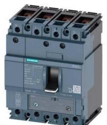
CIRCUIT BREAKER 3VA1 IEC FRAME 160 BREAKING CAPACITY CLASS M ICU=55KA @ 415 V 4-POLE, LINE PROTECTION TM240, ATAM, IN=16A OVERLOAD PROTECTION IR=11,2A ... 16A SHORT CIRCUIT PROTECTION II=5 X IN NEUTRAL PROTECTION 100% BUSBAR CONNECTION
