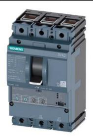
CIRCUIT BREAKER 3VA2 IEC FRAME 100 BREAKING CAPACITY CLASS C ICU=110KA @ 415 V 3POLE, LINE PROTECTION ETU330, LIG, IN=25A OVERLOAD PROTECTION IR=10A ...25A SHORT CIRCUIT PROTECTION II=1,5...12 X IN GROUNDFAULTPROTECTION IG=0,2... 1 X IN, TG=0,1/0,3MS CABLE CONNECTION
