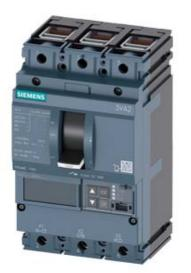
CIRCUIT BREAKER 3VA2 IEC FRAME 160 BREAKING CAPACITY CLASS C ICU=110KA @ 415 V 3POLE, LINE PROTECTION ETU560, LSIG, IN=160A OVERLOAD PROTECTION IR=64A ...160A SHORT CIRCUIT PROTECTION ISD=0,6..10X IN, II=1,5..10X IN NEUTRAL PROTECTION OPTIONAL WITH EXT. CT,UPTO 160% GROUNDFAULT, SWITCHABLE IG=0,2... 1 X IN, TG=0,050,8MS CABLE CONNECTION
