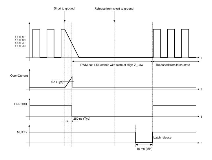
Figure 50. Output Short to GND Protection Sequence
