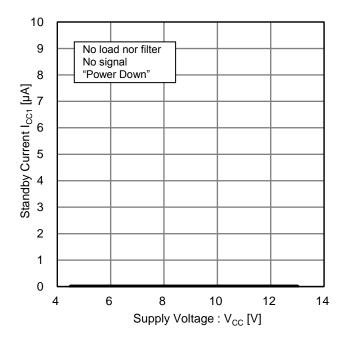
Figure 5. Standby Current vs Supply Voltage (Power Down)
