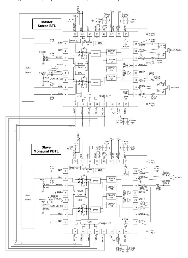
Figure 48. Application Circuit 5
