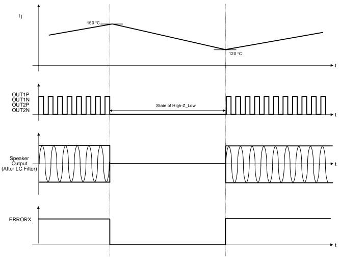
Figure 52. Overheat Protection Sequence
