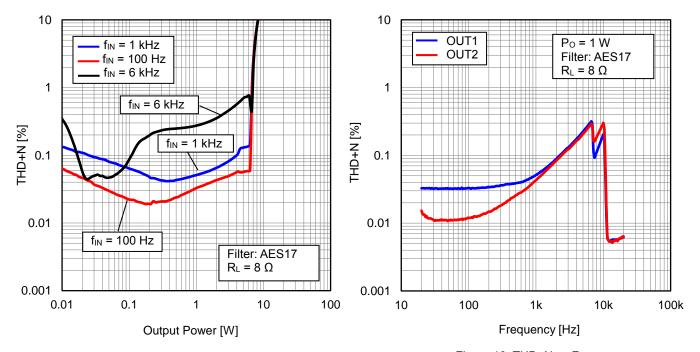
Figure 18. THD+N vs Output Power  $(R_L = 8 \Omega)$
