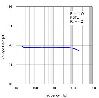
Figure 29. Voltage Gain vs Frequency (PBTL,  $R_L = 4 \Omega$ )
