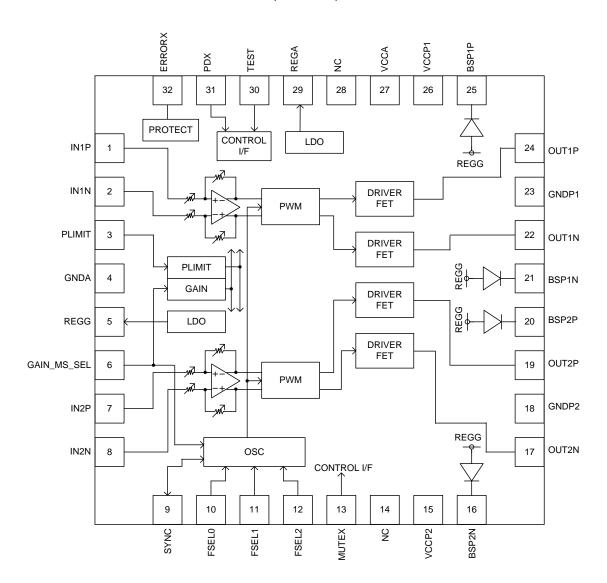
Figure 3. Block Diagram
