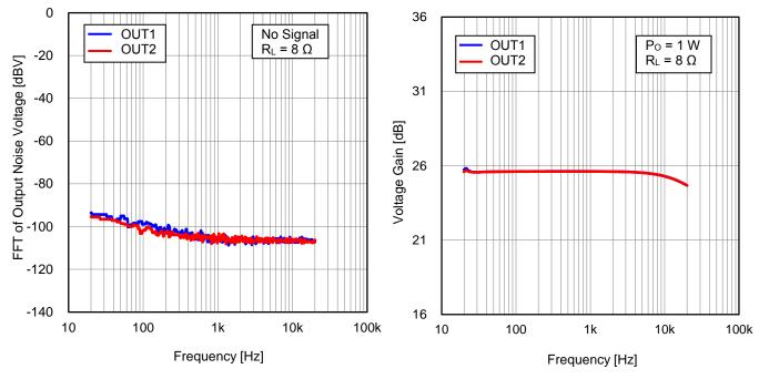
Figure 16. FFT of Output Noise Voltage vs Frequency (R<sub>L</sub> = 8  $\Omega$ )
