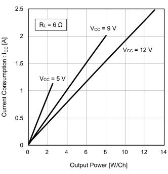
Figure 14. Current Consumption vs Output Power  $(R_L = 6 \Omega)$
