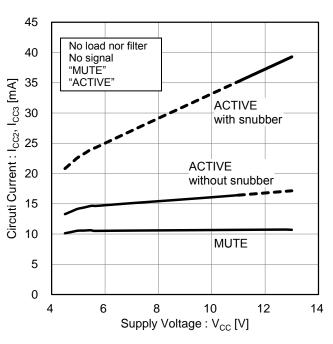
Figure 6. Circuit Current vs Supply Voltage (MUTE, ACTIVE)
