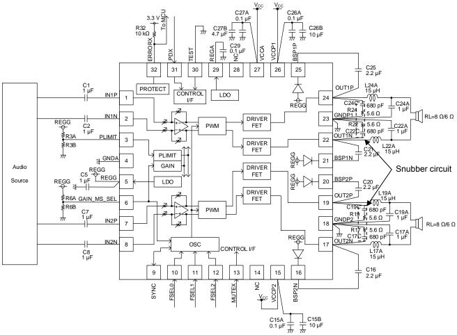
Figure 45. Application Circuit 2
