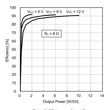
Figure 7. Efficiency vs Output Power ( $R_L = 8 \Omega$ )
