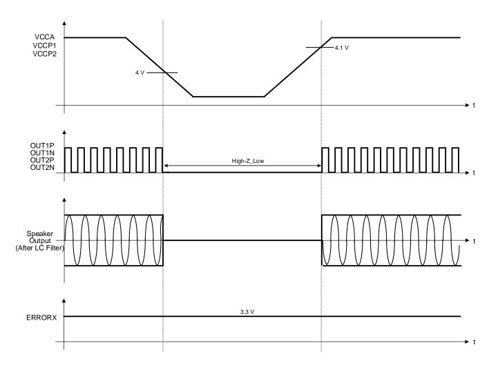
Figure 53. Under Voltage Protection Sequence
