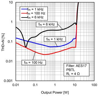
Figure 30. THD+N vs Output Power (PBTL,  $R_L = 4 \Omega$ )
