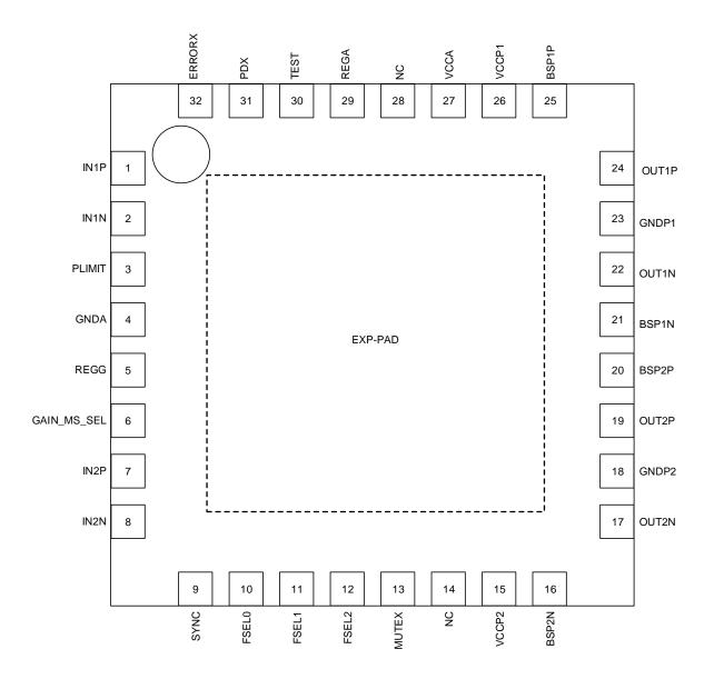
Figure 2. Pin Configuration
