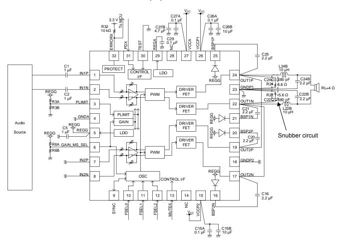
Figure 47. Application Circuit 4
