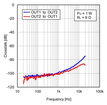
Figure 27. Crosstalk vs Frequency  $(R_L = 6 \Omega)$
