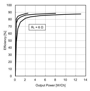
Figure 8. Efficiency vs Output Power  $(R_L = 6 \Omega)$
