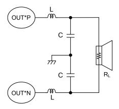
The following shows output LC filter constants and cutoff frequencies f<sub>C</sub> with typical load impedances.
