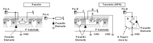
Figure 56. Example of monolithic LSI structure
