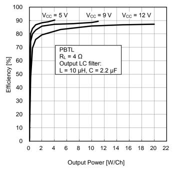
Figure 9. Efficiency vs Output Power (PBTL,  $R_L = 4 \Omega$ )
