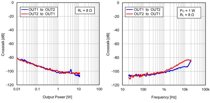
Figure 20. Crosstalk vs Output Power  $(R_L = 8 \Omega)$
