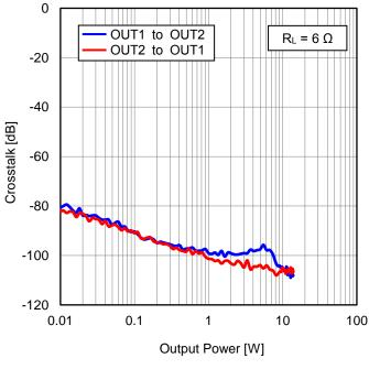
Figure 26. Crosstalk vs Output Power  $(R_L = 6 \Omega)$
