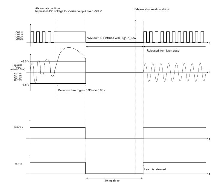
Figure 51. DC Voltage Protection at Speaker Sequence
