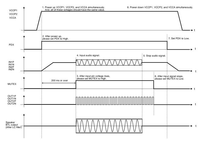
Figure 38. Power Up/Down Sequence
