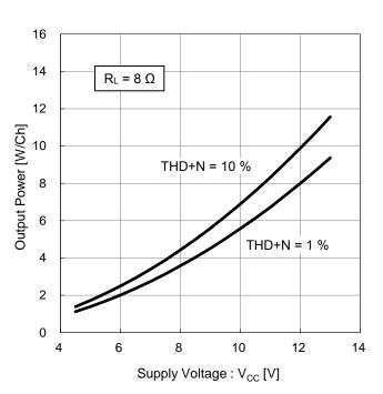
Figure 10. Output Power vs Supply Voltage ( $R_L = 8 \Omega$ )
