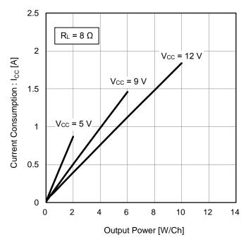
Figure 13. Current Consumption vs Output Power  $(R_L = 8 \Omega)$
