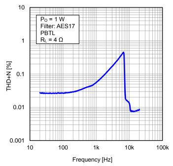
Figure 31. THD+N vs Frequency (PBTL,  $R_L = 4 \Omega$ )
