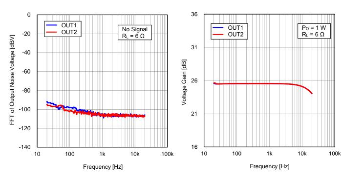
Figure 22. FFT of Output Noise Voltage vs Frequency  $(R_L = 6 \Omega)$
