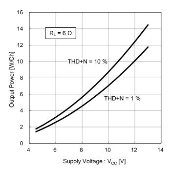
Figure 11. Output Power vs Supply Voltage  $(R_L = 6 \Omega)$
