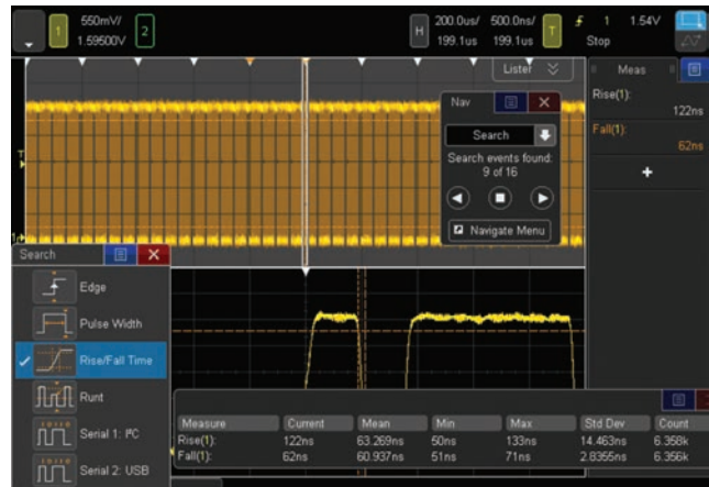
Figure 10a. The 4000 X-Series was set up to capture data signals with various rise time edges. Using the search and navigation capability, the oscilloscope was able to find, mark (white triangles), and quickly navigate to 16 occurrences of "out of compliance" rise-time edges.
