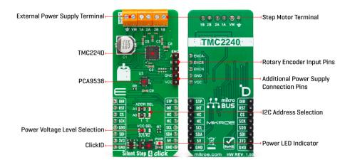
One cool feature is the rotary encoder interface integration directly into the step driver. The external incremental encoder can be connected over the ENC connector. The encoder can be used for consistency checks on the fly between the encoder position and the external ramp generator position. A 32-bit encoder counter is provided. StallGuard2 is a great functionality for detecting a motor stall and is part of the diagnostic system of the stepper driver.
