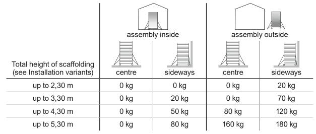
Ballast weights can be attached to the outrigger. Arrange the ballast weights symmetrically. When arranged sideways, the weights must be hooked onto the long side, as far out as possible.
