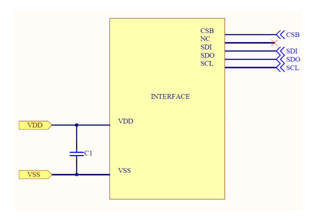
Pin connected to MCU interface: CSB,SDI,SDO,SCL
