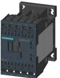
COUPLING RELAY, AC-3, 3KW/400V, 1NC, DC 12V, 0.7...1.25\*US, W. PLUGGED-ON VARISTOR 3-POLE SZ S00, SPRING-LOADED TERMINAL
