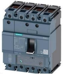
CIRCUIT BREAKER 3VA1 IEC FRAME 160 BREAKING CAPACITY CLASS N ICU=25KA @ 415 V 4-POLE, LINE PROTECTION TM240, ATAM, IN=100A OVERLOAD PROTECTION IR=70A ...100A SHORT CIRCUIT PROTECTION II=5...10 X IN NEUTRAL PROTECTION 50% CABLE CONNECTION
