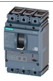
CIRCUIT BREAKER 3VA2 IEC FRAME 160 BREAKING CAPACITY CLASS C ICU=110KA @ 415 V 3POLE, LINE PROTECTION ETU330, LIG, IN=100A OVERLOAD PROTECTION IR=40A ...100A SHORT CIRCUIT PROTECTION II=1,5...12 X IN GROUNDFAULTPROTECTION IG=0,2... 1 X IN, TG=0,1/0,3MS CABLE CONNECTION
