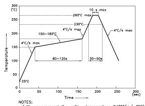
NOTES: 1.We recommend the reflow temperature 245°C(+/-5°C).The maximum soldering temperature should be limited to 260°C. 2.Don't cause stress to the epoxy resin while it is exposed to high temperature. 3.Number of reflow process shall be 2 times or less.
