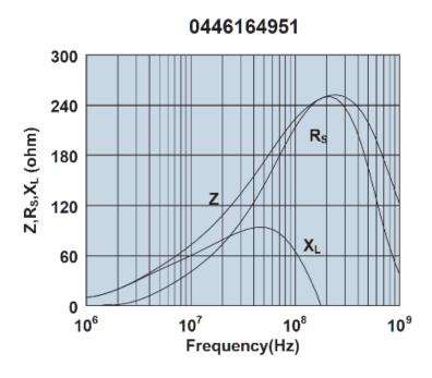
Impedance, reactance, and resistance vs. frequency.
