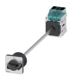
Switch disconnector 3LD3, main switch 3-polig, lu 40A operational switch at AC-23 A at 400 V 15,0 kW floor mounting Base mounting with door coupling center-hole 22,5 mm knob-operated mechanism black 48 x 48 mm with auxiliary 1NO+1NC
