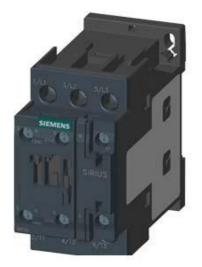
CONTACTOR, AC-3, 15KW/400V, 1NO+1NC, AC 48V 50/60HZ, 3-POLE, SZ S0 SCREW TERMINAL
