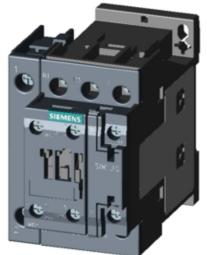
2NO+2NC CONTACTOR, AC3: 11KW AC 24V 50/60HZ 4-POLE, 2NO+2NC, SZ: S0, SCREW TERMINAL 1NO+1NC INTEGR.
