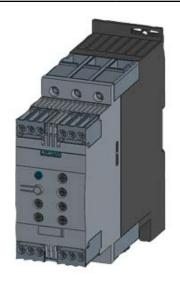
SIRIUS SOFT STARTER, S2, 45A, 30KW/500V, 40 DEGR., AC 400-600V, AC/DC 24V, SCREW TERMINALS
