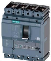
CIRCUIT BREAKER 3VA2 IEC FRAME 100 BREAKING CAPACITY CLASS L ICU=150KA @ 415 V 4POLE, LINE PROTECTION ETU330, LIG, IN=25A OVERLOAD PROTECTION IR=10A ...25A SHORT CIRCUIT PROTECTION II=1,5...12 X IN NEUTRAL PROTECTION ADJUSTABLE(OFF,100%) GROUNDFAULTPROTECTION IG=0,2... 1 X IN, TG=0,1/0,3MS BUSBAR CONNECTION
