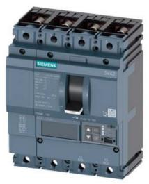
CIRCUIT BREAKER 3VA2 IEC FRAME 160 BREAKING CAPACITY CLASS L ICU=150KA @ 415 V 4POLE, LINE PROTECTION ETU550, LSI, IN=40A OVERLOAD PROTECTION IR=16A ...40A SHORT CIRCUIT PROTECTION ISD=0,6..10X IN, II=1,5..12X IN NEUTRAL PROTECTION ADJUSTABLE (OFF, UPTO 160%) BUSBAR CONNECTION
