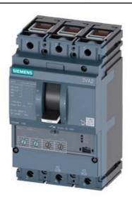
CIRCUIT BREAKER 3VA2 IEC FRAME 160 BREAKING CAPACITY CLASS M ICU=55KA @ 415 V 3POLE, LINE PROTECTION ETU330, LIG, IN=63A OVERLOAD PROTECTION IR=25A ...63A SHORT CIRCUIT PROTECTION II=1,5...12 X IN GROUNDFAULTPROTECTION IG=0,2... 1 X IN, TG=0,1/0,3MS CABLE CONNECTION
