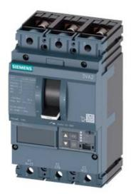
CIRCUIT BREAKER 3VA2 IEC FRAME 160 BREAKING CAPACITY CLASS H ICU=85KA @ 415 V 3POLE, LINE PROTECTION ETU850, LSI, IN=63A OVERLOAD PROTECTION IR=25A ...63A SHORT CIRCUIT PROTECTION ISD=0,6..10X IN, II=1,5..12X IN NEUTRAL PROTECTION OPTIONAL WITH EXT. CT,UPTO 160% BUSBAR CONNECTION
