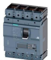
CIRCUIT BREAKER 3VA2 IEC FRAME 400 BREAKING CAPACITY CLASS H ICU=85KA @ 415 V 4-POLE, LINE PROTECTION ETU560, LSIG, IN=250A OVERLOAD PROTECTION IR=100A ...250A SHORT CIRCUIT PROTECTION ISD=0,6..10X IN, II=1,5..12X IN NEUTRAL PROTECTION ADJUSTABLE (OFF, UPTO 160%) GROUND-FAULT, SWITCHABLE IG=0,2... 1 X IN, TG=0,05-0,8MS BUSBAR CONNECTION
