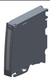
SIMATIC S7-1500, ANALOG OUTPUT MODULE AQ 2 X U/I ST; 16 BITS OF RESOLUTION, ACCURACY 0.3 %; 2 CHANNELS IN GROUPS OF 2; DIAGNOSIS, SUBSTITUTE VALUE INCL. FRONT CONNECTOR PUSH-IN, FEEDING ELEMENT, SHIELDING ELE-MENT, SHIELDING CLAMP
