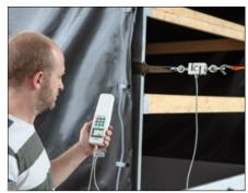
Universal digital force gauge for tensile and compressive force measurements with external load cell
