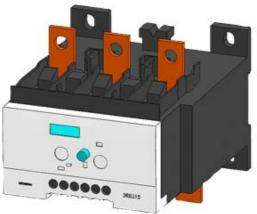
OVERLOAD RELAY 50...200 A FOR MOTOR PROTECTION SIZE S6, CLASS 5...30 MOUNT. ONTO CONT./ STAND-ALONE MAIN CIRCUIT: BAR CONNECTION AUX. CIRCUIT: SCREW CONNECTION MANUAL-AUTOMATIC-RESET INT. EARTH FAULT DETECTION
