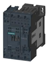
4NO CONTACTOR, AC1: 35A DC 110V 4-POLE, 4NO, SZ: S0, SPRING-LOADED TERMINAL 1NO+1NC INTEGR.
