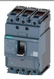
CIRCUIT BREAKER 3VA1 IEC FRAME 160 BREAKING CAPACITY CLASS S ICU=36KA @ 415 V 3-POLE, LINE PROTECTION TM220, ATFM, IN=160A OVERLOAD PROTECTION IR=112A ...160A SHORT CIRCUIT PROTECTION II=10 X IN CABLE CONNECTION
