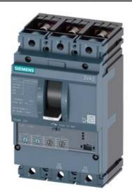
CIRCUIT BREAKER 3VA2 IEC FRAME 250 BREAKING CAPACITY CLASS H ICU=85KA @ 415 V 3POLE, LINE PROTECTION ETU330, LIG, IN=250A OVERLOAD PROTECTION IR=100A ...250A SHORT CIRCUIT PROTECTION II=1,5...10 X IN GROUNDFAULTPROTECTION IG=0,2... 1 X IN, TG=0,1/0,3MS BUSBAR CONNECTION
