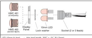
LED 10mm bi-lead - trim lead length  $.300" \pm .01"$  (8.13mm) Panel Thickness - .032" to .187", Panel Hole: .562" (14.0mm)
