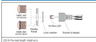
LED Hi-Flux lead length: Install as is. Panel thickness - .032" to .187" Panel Hole: .562" (14.0mm).
