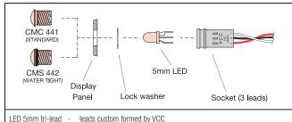
LED 5mm tri-lead - leads custom formed by VCC
