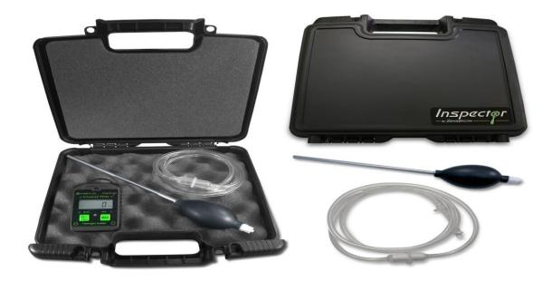
Description: Sensorcon proudly presents the **Industrial Pro Hydrogen Sulfide Detector!** A wearable, programmable, and realtime display H2S detector for the modern work force. Set your own alarm points to meet your specific industry needs! This Inspector's professional feature highlights include:
