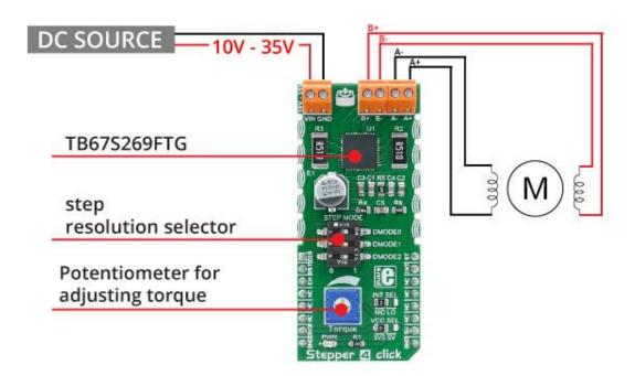
The other four connectors are used for connecting the stepper motor to the click. After a motor is connected, it can be controlled by the MCU through the Stepper 4 click.
