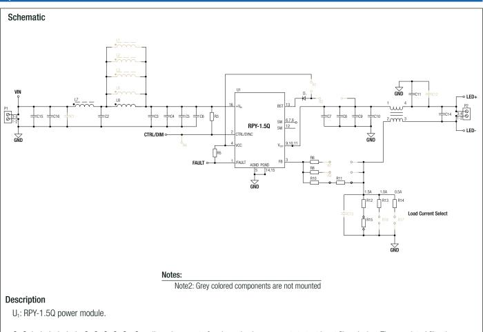
$C_{1}$ ,  $C_{2}$ ,  $L_{1}$ ,  $L_{2}$ ,  $L_{3}$ ,  $L_{6}$ ,  $L_{7}$ ,  $L_{8}$ ,  $C_{3}$ ,  $C_{4}$ ,  $C_{5}$ ,  $C_{6}$ ,  $C_{15}$ ,  $C_{16}$ : allow placement of various sized components to test input filter design. The populated filter is designed to meet CISPR25 Class 5.
