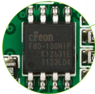
Figure 11-1: Flash memory module
