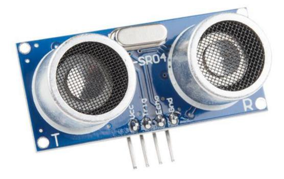
This is the HC-SR04 ultrasonic distance sensor. This economical sensor provides 20 mm to 4 m of non-contact measurement functionality with a ranging accuracy that can reach up to 3mm. Each HC-SR04 module includes an ultrasonic transmitter, a receiver and a control circuit.
