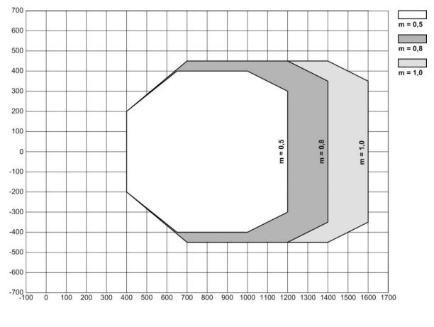
Reading field distance [mm] Reading field width [mm] Х
