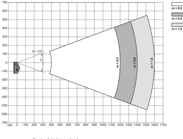
x Reading field distance [mm] y Reading field height [mm]
